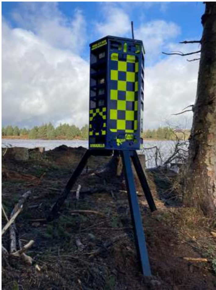
Figure 3. One of two intrusion detection cameras installed near the nest.
